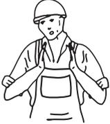
A line drawing of a worker wearing a hard hat and a work shirt. The worker is holding both hands parallel to each other, palms facing each other, at chest level. The hands are held close together, indicating a specific distance or a reduction in distance.                                | Beide Handflächen parallel dem Abstand entsprechend halten. |
