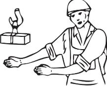
A line drawing of a worker wearing a hard hat and a work shirt. The worker is pointing with both hands towards a small rectangular object on a stand to their left. The worker's right hand is extended forward, and the left hand is also extended forward, both pointing towards the object. | Mit beiden Händen auf Zielpunkt zeigen.                     |
