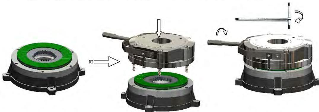
6. Adjust the air gap (the red coloured area) to the value shown in the specification working on the fixing screws and the adjusting nuts as follows:
