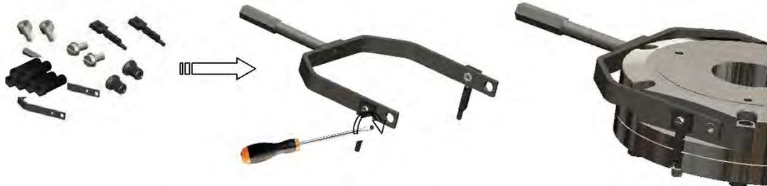
5. To place the disc brake on the shield of the motor. Then fix the brake unit tightening the screws.
