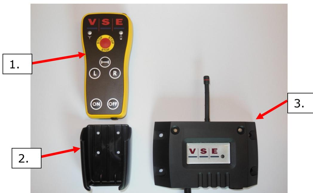
It is recommended that the holder (2) be installed in an easily accessible location (such as in the cab of the truck) and that the handset be placed in the holder when not in use.
