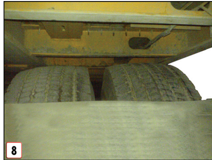
8 Because of excessive load the distance between the rear wheels and the crosses in the king pin area is too small. During the extension operation the air bellows cannot accomplish their task as suspension.
